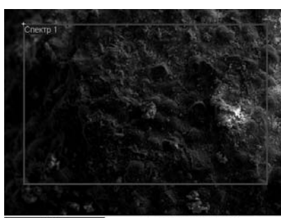
Fig. 4. SEM image of magnesite waste. The elemental composition of the X-ray part of the spectrum, designated as “Spectrum 1”: O – 60, Mg – 27, Si – 8, Ca – 5, Fe – 1 %.
