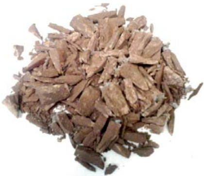
Fig. 8. The destruction nature of the sample with 5 % magnesite waste. Firing temperature = 1150 °C. Compressive strength – 148 MP.
