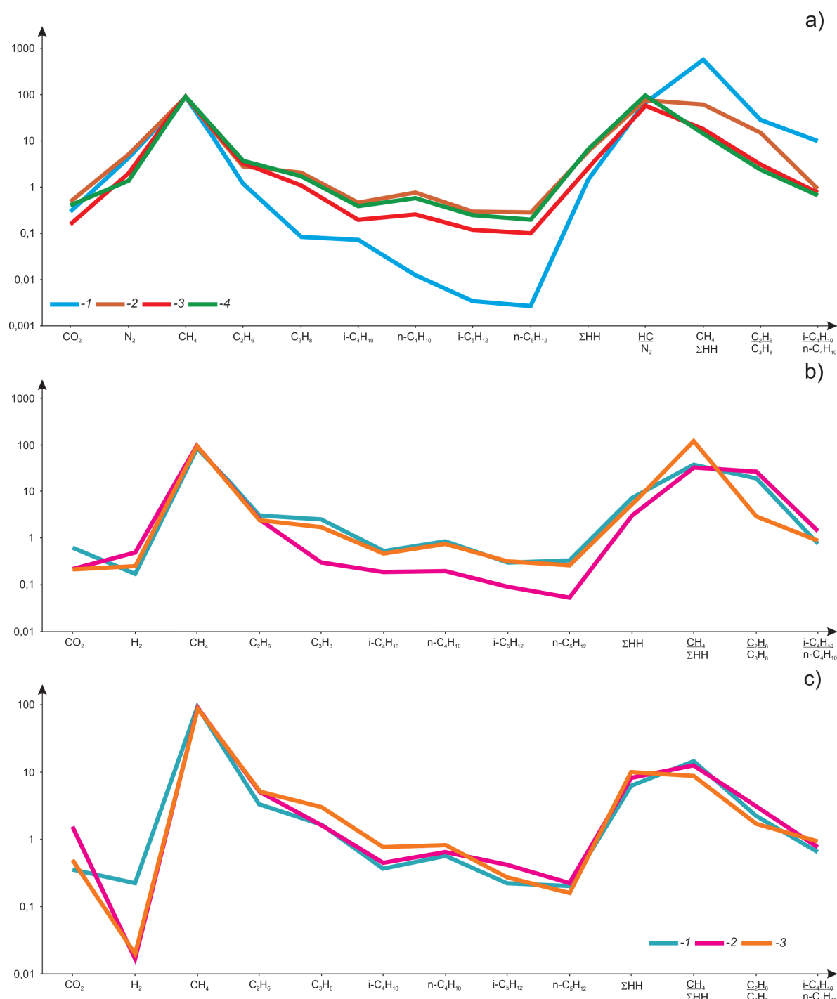
Fig. 3. Average composition of the WDG of oil and gas bearing sediments in the junction of the Yenisei-Khatanga and the West Siberian basins taking into account the main geochemical coefficients ( CH_4/\Sigma TV , C_2H_6/C_3H_8 and i-C_4H_{10}/n-C_4H_{10} ): a) aquifer systems: 1 – the Aptian-Albian-Cenomanian, 2 – the Neocomian, 3 – the Upper Jurassic, 4 – the Lower and Middle Jurassic; b-c) the studied regions: 1 – the Yenisei-Khatanga basin, 2 – the Messoyakh inclined ridge, 3 – the West Siberian basin.
