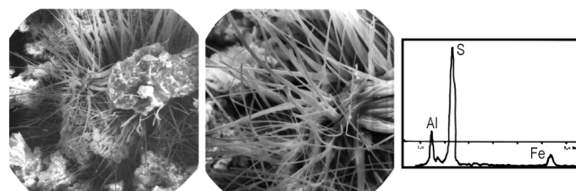
Fig. 6. Left to right: Hair-like crystals of iron-aluminum alum in the rocks of Bazhenov formation, magn. 300 x . Fragment of the previous image, magn. 1000 x . Energy-dispersive spectrum of crystals of iron-aluminum alum: Al, S, Fe
