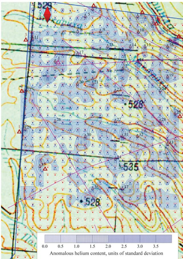
Fig. 2. Topographic base fragment of the helium survey site with its results,  $\blacklozenge$  – a drilled search well that gave the gas inflow from the Yarakhtinskian horizon
