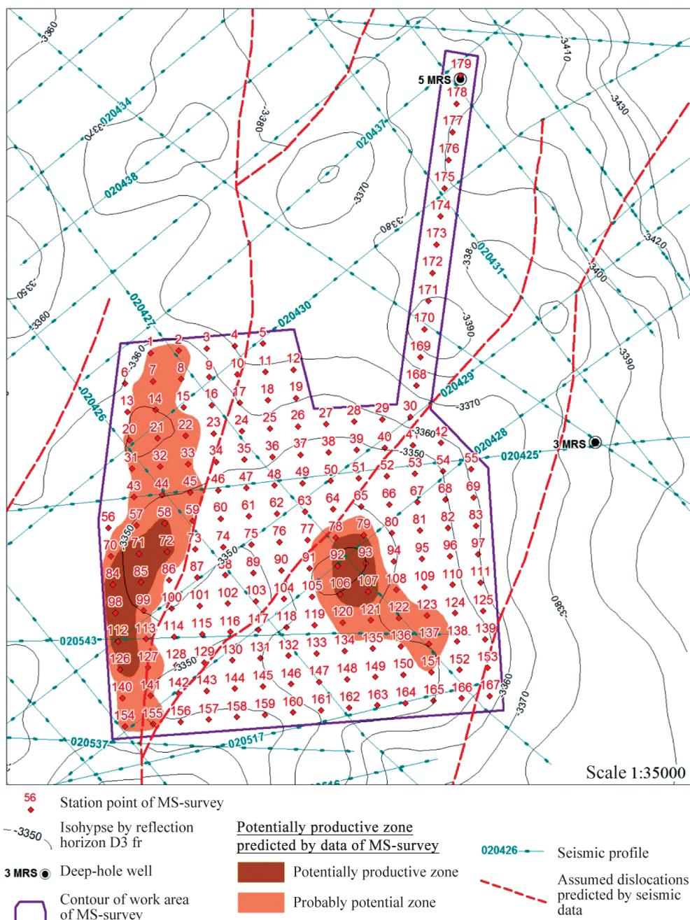
Fig. 5. A productive well No. 32 was drilled near the point No. 71 of the MS field survey
