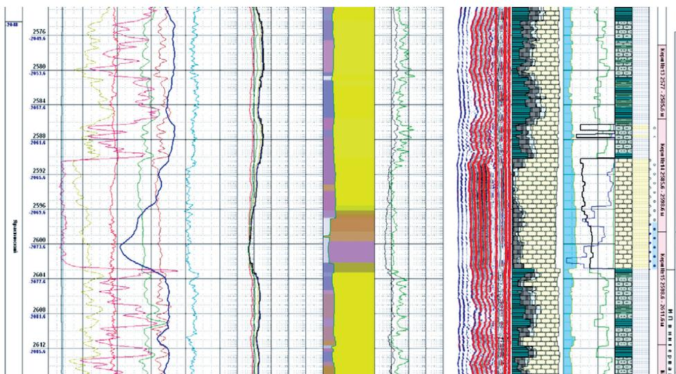
Fig. 4. According to the logging, the Yarakhtinskian horizon of the search well in the depth interval 2590-2596 m is gas-saturated
