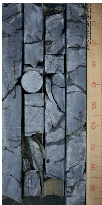
Fig. 1. Fractured core from well 181 VIU. Interval 1864-1869 m
