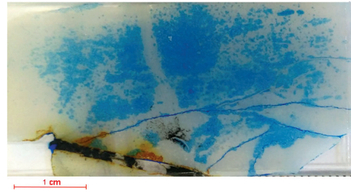
Fig. 5. Uneven saturation by colored epoxy resin (blue color is porous part). Fracture with bituminous filling. A sample from the well of the Sovetsko-Kurskaya area (depth of 3463.33 m). Thin section photo.
