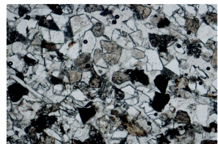
Fig. 4. Sandstone fine, arkose with uniform pore basal carbonate cement. View – under crossed nicols, increase of 100X, sample 15620-08, interval 2073-2080 m, sampling point 1.58 m. Malokhetskian Formation, layer Mkh-III, well Tgl-4. biotite in the stage of early amorphization.
