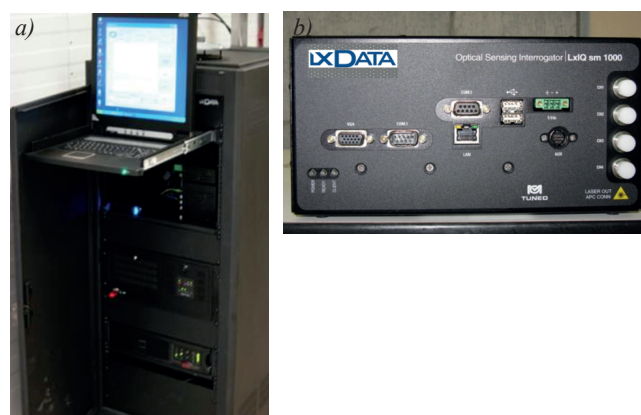
Fig. 9. Hardware rack of the control center (a) and control panel (b) of 19" size ( www.weatherford.com )
