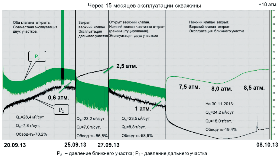
Fig. 4. Dynamics of bottomhole pressures and liquid production rates after switching flow regulation valves for well 41502G
