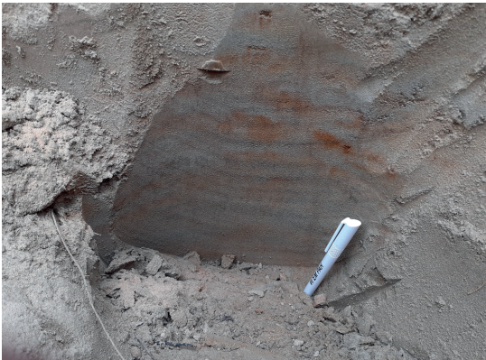
Fig. 3. Productive layer of the Itmanovs placer: dark interlayers contain increased concentrations of ore minerals – ilmenite, chromite and zircon
