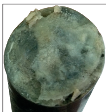
Fig. 8. Crystal formation of magnesium chloride on the stone surface
