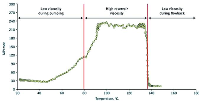
Fig. 9. Dependence of the acid viscosity on temperature (Guo Jian-Chun, Gou Bo, Yu Ting, 2015)
