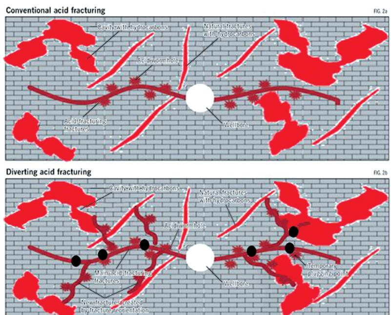
Fig. 8. Normal (a) and deflecting (b) acid fracturing (Guo Jian-Chun, Gou Bo, Yu Ting, 2015)
