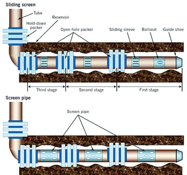
Fig. 10. Methods of separate completion of horizontal well in acid fracturing in an open trunk (Guo Jian-Chun, Gou Bo, Yu Ting, 2015)
