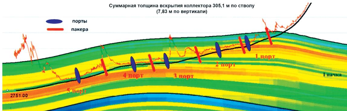
Fig. 3. Geological section within the horizontal section of the trunk of well 310 Rechitsky (Demyanenko, Serebrennikov, Povzhik et al., 2017)
