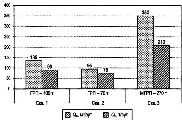
Fig. 6. Comparative results of standard hydraulic fracturing and multiple hydraulic fracturing for liquid and oil flow rates: Well 1 – controlled directional well with a standard fracturing of 100t proppant; Well 2 – controlled directional well with a standard fracturing of 70t proppant; Well 3 – horizontal well with a multiple fracturing performed with a total volume of 270 t proppant (Shirokov, Azamatov, Artamonova, 2013)
