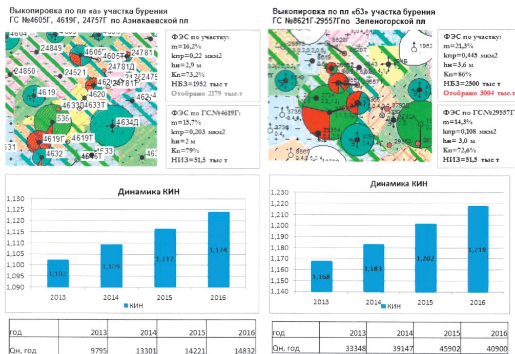
Fig. 2. Dynamics of oil recovery factor for horizontal wells with "off-balance" production of reserves (Taipova, 2016)
