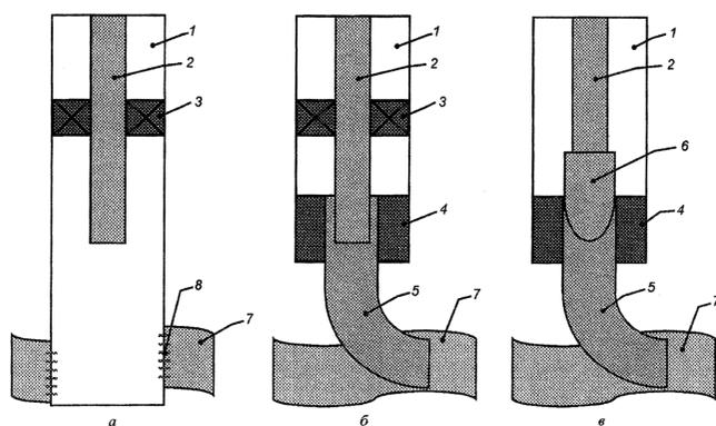
Fig. 5. Scheme of descent of underground equipment for standard hydraulic fracturing on a controlled directional well (a), standard hydraulic fracturing on a horizontal well (b) and multiple hydraulic fracturing on a horizontal well (c). 1 – the main production column; 2 – tubing string; 3 – hydraulic fracturing packer; 4 – liner hanger; 5 – shank; 6 – stinger; 7 – reservoir; 8 – interval of perforation (Shirokov, Azamatov, Artamonova, 2013)
