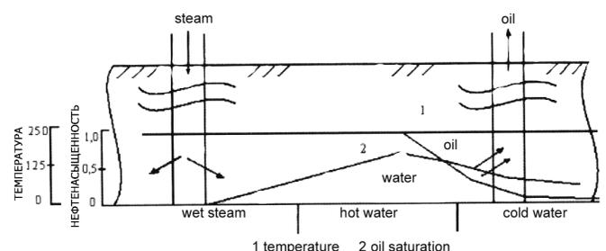
Fig. 1. Continuous steam injection scheme (Gataullin, Marfin, Kokhanova, 2007)
