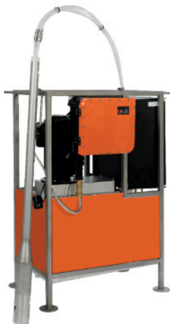
Fig. 7. Complete mud gas system. Note the extraction probe, and the complete system being a stand alone system, safe to be used directly near the shale shakers or flowline
