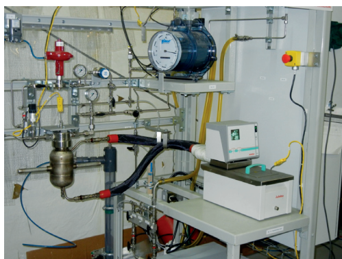
Figure 15. Isothermal Cell for Studying Kinetics of Oxidation
