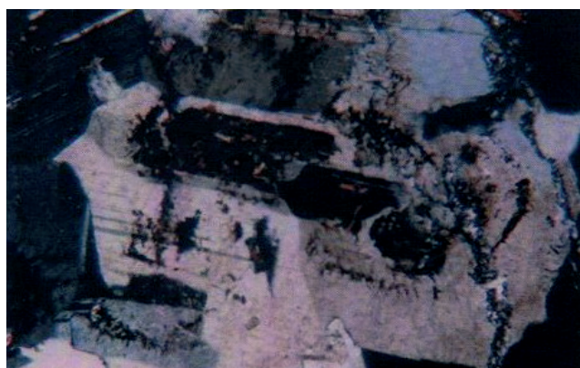
Fig. 3. Granite. Dark brown bitumen in the leaching pores in plagioclase. Increase × 40 Nicoli + Depth 4307 m, Well BT 448.
