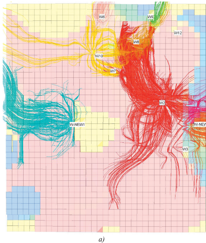
Figure 11. Filtration lines of oil flow in the Bobrikovian object (incision): a) 1 option without reservoir pressure maintenance, b) 2 option with reservoir pressure maintenance
